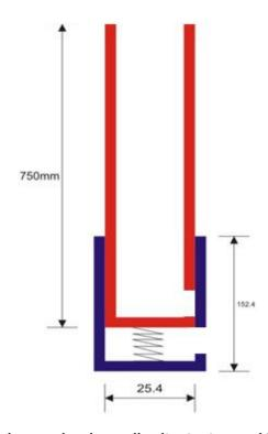
The above elements are assembled in such a way that the smaller dia pipe is seated in larger dia pipe so it can slide into it, the sliding pin passed through pipe via slot to constrain the relative motion of pipe and a backthrust is obtained using compression spring placed below.
